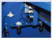
Nozzle selection Right and/or left, for a better spraying precision and no waste of pretreatment liquid.
